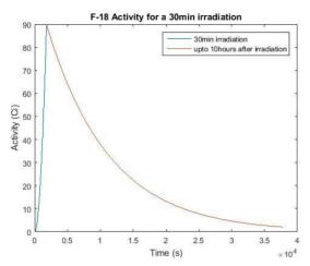
Figure 6: Activity of F-18obtainable using QGSP\_BIC\_AllHP.
