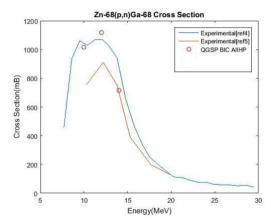
Figure 1: Experimental and simulated cross section results for the production of Ga-68 [5,6].
