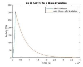
Figure 4: Activity of Ga-68 obtainable using QGSP\_BIC\_AllHP
