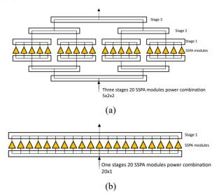
Figure 3: (a) SSPAs are grouped in sets of five and combined twice in three stages 5x2x2 (b) SSPAs are combined only once as a 20x1 combination.
