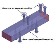
Figure 7: Expandable 2-stage coaxial-to-waveguide power combiner.
