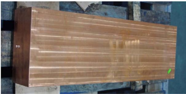
Figure 2: Squared block for a major vane fabrication. Holes to guide the deep drilling of the cooling channels are also shown.
