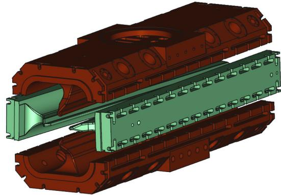
Figure 1: Exploded view of first segment of the RFQ, separated in two major and two minor vanes.
