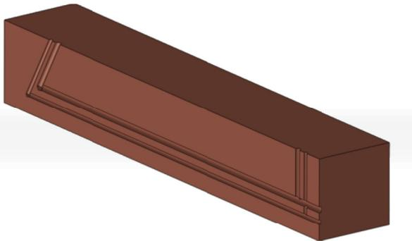
Figure 3: Model showing the deep drilling of the longitudinal cooling channels.
