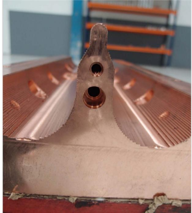
Figure 4: A major vane after rough machining. The holes of the cooling channels can be seen in the vane.
