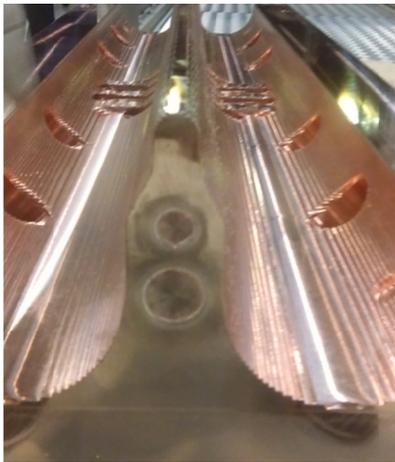
Figure 5: A major vane after cooling channels plugs have been inserted and welded by EBW.
