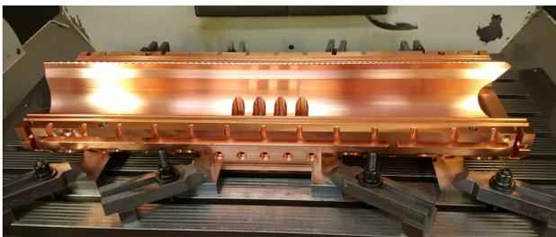
Figure 6: A major vane of the RFQ after fine machining in the milling machine.
