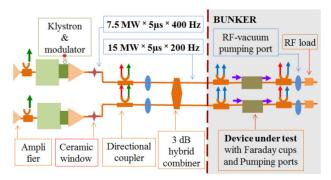
Figure 1: Layout of the high-power subsystem of the IFIC HG RF laboratory.
