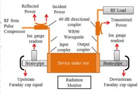
Figure 5: Schematic layout of the device under test and the various diagnostic systems. The red arrows show the
