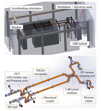
Figure 2: 3D design of the high-power network of the IFIC HG RF laboratory. Top picture: integration in the laboratory enclosure of the building. Bottom picture: detail of the assembly of the high-power and vacuum components from the klystron output.
