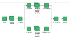
Figure 1: The schematic of 24KW solid-state amplifier (the pre-amplifier as Fig. 2 and the main amplifier an Fig. 3).
