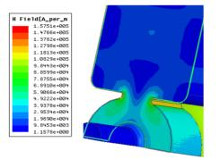
Figure 10: The peak magnetic field at the coupler windows.
