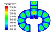
Figure 8: The electromagnetic distribution of the splitter.
