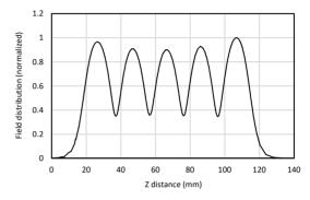
Figure 9 (c): The field distribution along axis.
