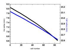
Figure 4: Each cavity's iris and cell radius.
