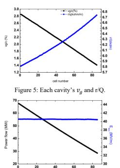
cell number Figure 6: The power flow and  $E_{acc}$  along the structure.
