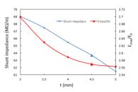
Figure 1: The shunt impedance and  $\text{Emax}/\text{E}_0$  VS. disk thickness t.
