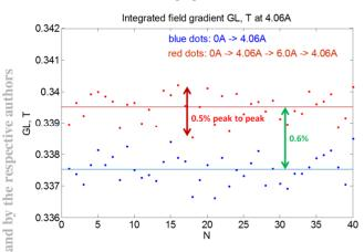
Figure 6: Integrated gradient of 40 QM2 quadrupoles measured with the rotating coil. The measurement allows estimating the spread of the quads strength and importance of the special turn-on procedure, which is chosen as increasing the current to 6.0 A and reaching the set value afterwards from above.
