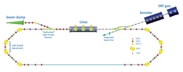
Figure 1: Layout of the bERLinPro magnetic system.
