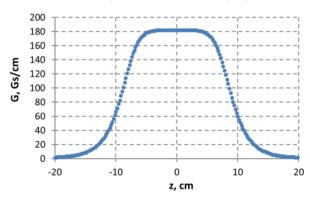
Figure 2: Gradient profile of a QM2 magnet derived from the Hall probe measurement. z is the coordinate along the beam axis.
