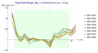
Figure 4: Homogeneity of magnetic field in the centre (z) of 8 BM3 magnets, measured with 16 Hall probes. The field is normalised to the central (x = 8 cm) Hall probe. Good field region ( $\Delta B = 4$  Gs,  $\Delta x = 13$  cm, shown as green rectangle) is within specification. Probe to probe systematic error of ~ 0.3‰ can be seen.
