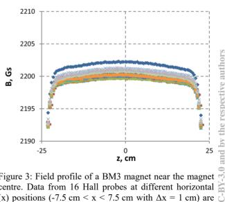
Figure 3: Field profile of a BM3 magnet near the magnet centre. Data from 16 Hall probes at different horizontal (x) positions (-7.5 cm < x < 7.5 cm with  $\Delta x = 1$  cm) are shown.
