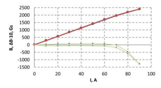
Figure 5: Hysteresis curve of a BM3 magnet. Field in the magnet centre for increasing current from 0 A to 90 A in 10 A steps is shown with red markers, for decreasing current – with blue. Green line shows the difference between the measured field and a straight line (multiplied with 10 for visualisation). Slight saturation is seen and can be accounted for during operation.
