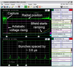
Figure 4: Upper plot: LLRF signals on injection plateau. Traces: magnetic field (yellow); measured radial position (green); detected HLRF voltage (pink); frequency program (blue). Lower plot: bunched beam on a shorter time-scale.
