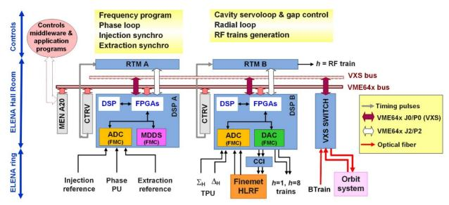
Figure 2: ELENA LLRF schematic view. Keys: MDDS – Master Direct Digital Synthesiser; ADC – Analogue-to-Digital Converter; DAC – Digital-to-Analogue Converted; TPU – Transverse Pick-up; CTRV – Timing Receiver Module; MEN A20 – Master VME board; RTM – Rear Transition Module; CCI – Cavity Control Interface.
