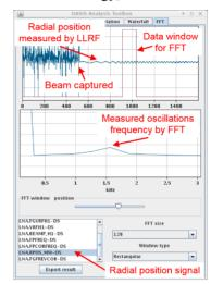
Figure 5: Synchrotron frequency obtained by FFT of radial position oscillations as measured by the LLRF system.
