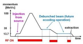
Figure 1: Qualitative view of an ELENA cycle for commissioning when beam is injected from the H<sup>-</sup> source. The red RF segments show when the LLRF voltage is active.
