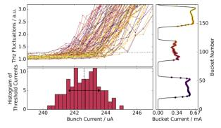
Figure 3: THz fluctuations as function of bunch current for all bunches in a multi-bunch fill. The vertical (doted) line in the histogram of the threshold currents of each bunch (lower panel) indicates the average of the threshold currents  $\mu(I_{\rm th})$ while the horizontal arrows indicate the spread (standard deviation) of threshold currents  $\sigma$  ( $I_{\rm th}$ ). The filling pattern at the start of the decay is indicated in the right plot.
