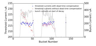
Figure 2: Threshold current per bunch as function of bunch number. Due to the dead time effect the bunch current is determined falsely, leading to differences in the threshold currents (in red). The systematic in the differences originates from the combination of the dead time duration of 87 ns (44 buckets) and the filling pattern (in grey). After the compensation of the dead time effect the systematic differences vanish and the spread decreases (in blue).
