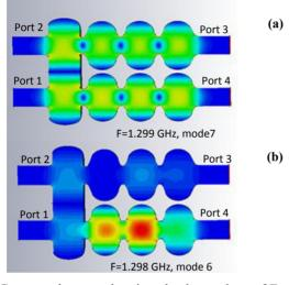
Figure 2: Contour plots are showing absolute values of Efield distributions for (a) operating mode at 1.299 GHz and (b) asymmetric mode at 1.298 GHz.
