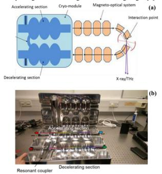
Figure 1: (a) Schematic diagram of the SCRF ERL system proposed to generate high luminosity photons [2]. (b) photograph of the 7-cell aluminium cavity.
