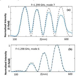
Figure 4: The graph are illustrating the normalized field intensity of the operating mode (a) and the nearest mode with the highest Q-factor (b) along axis 1 as measured (solid lines) and calculated (dashed lines) using CST MW studio.
