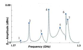
Figure 3: Graph illustrating  $S_{41}$  parameter as measured (solid line) between ports 1 and 4 in the frequency range from 1.27 GHz to 1.305 GHz and predicted using coupled modes (Fano) approximation (dashed line). The solid dot at the  $S_{41}$  maxima illustrates the position of the eigenmodes as predicted by the CST MW studio.
