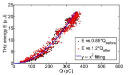
Figure 4: Measured THz energy varies as the effective charge. The definition of the effective charge  $(0.85*Q_{before}$  or  $1.2*Q_{after})$  depends on the measurement of THz energy versus the charge compared with the coherent radiation curve ( $y \propto x^2$ ).
