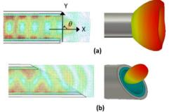
Figure 1: The electric field and the far-field distribution of  $TM_{01}$  mode at the end of the DLW without angle cut, and as well as the ones in the DLW with an angle cut.
