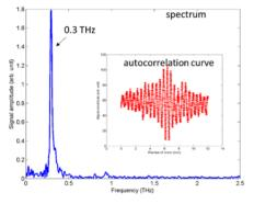
Figure 5: The autocorrelation curve from the interferometer and the spectrum of the 300 GHz DLW.
