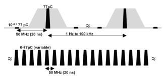
Figure 2: Pulse patterns during initial commissioning with the 50 MHz laser. The laser will be able to produce single bunches at a variable rate of 1 Hz to 100 kHz (SB mode, top) or continuous 50 MHz bunches (CW mode, bottom).
