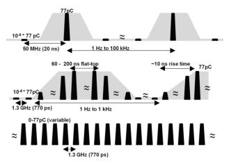
Figure 3: Pulse patterns after the 1.3 GHz laser is installed. The 50 MHz laser will produce single bunches at a variable rate of 1 Hz to 100 kHz (SB mode, top), and the 1.3 GHz laser will produce macro-pulses of 1.3 GHz bunches at a variable rate of 1 Hz to 1 kHz (MP mode, center) or continuous 1.3 GHz bunches (CW mode, bottom).
