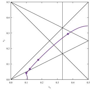
Figure 5: Tune per cell for the arc cell, treated as periodic. Design energies are shown with dots.
