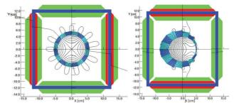
Figure 3: The cross sections of the (QF) a pure focusing Halbach magnet (left), and the (BD) a defocusing quadrupole magnet with a dipole component (right). Both QF and BD Halbach magnets have window frame electromagnets as correctors.
