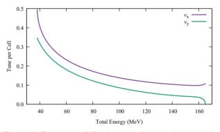
Figure 6: Tune per cell for the arc cell, treated as periodic, as a function of energy.
