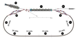
Figure 1: Layout of the CBETA accelerator. The section labeled (LA) is the ERL, The sections labeled (FA), (TA), (ZA), (ZB), (TB), and (FB) are the FFAG sections which accommodate four recirculating electron bunches which have an energy range from 42 MeV to 150 MeV.
