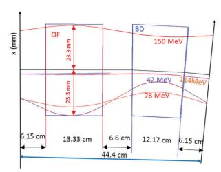
Figure 2: A schematic diagram of the FFAG doublet cell showing the trajectories of the electron bunches ranging in energy from 42 to 150 MeV in constant magnetic field. The label QF designates the pure focusing quadrupole and the label BD the defocusing quadrupole with the dipole component.
