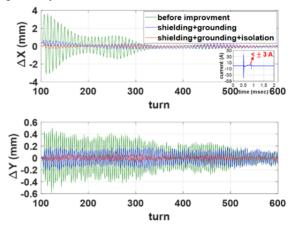
Figure 5: Turn-by-turn BPM data with best matched kicker show betatron oscillations before improvement (green), after mu-metal shielding and grounding with copper cables (blue) and after isolation of current loops (red). The figure insert shows the eddy current after improvements.
