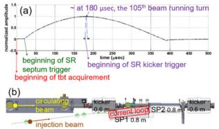
Figure 2: (a) time-relation scheme of septum (black) and kicker magnets (blue), (b) layout of the injection section.
