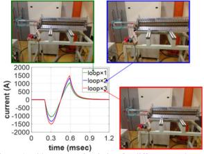
Figure 4: eddy current simulation for different numbers of parallel current loops.
