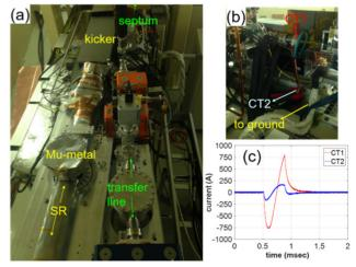
Figure 3: (a), (b) photos of the injection section and (c) eddy current measurements in the real machine.
