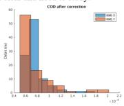
Figure 5: Distribution of rms orbit after correction (100 seeds).
