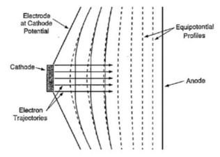
Figure 2: Schematic of the flat cathode pierce electron gun.
