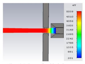
Figure 4: Trajectory of particles in the gun.
