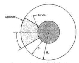
Figure 1: Structure of a spherical cathode electron gun.
