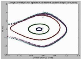
Figure 3: beam longitudinal phase space at different RF phase jump amplitude.
