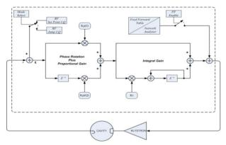
Figure 1: Schematic of NSLS-II cavity field controller.
