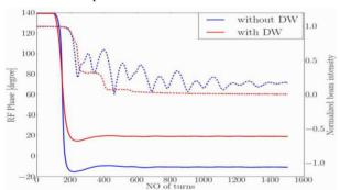
Figure 4: RF momentum aperture measurement without and with DW.
