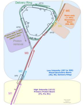
Figure 1: Schematic illustration of the Muon Campus beamlines. Devices will be distributed along the Muon Campus based on beam intensity. More details can be found in Ref. 3.
