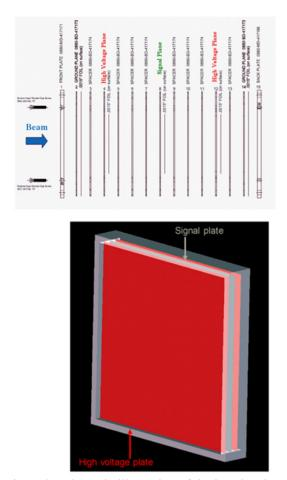
Figure 2: Schematic illustration of the ion chamber detector. The bottom figure shows the simulation model.
