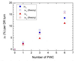
Figure 4: Horizontal and transverse emittance growth vs the number of PWCs along the beamline. Open symbols are results from theory while solid symbols are results from simulation.
