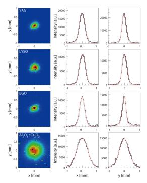
Figure 3: Background corrected beam images and projected beam profiles at 1 nC/bunch beam (single shot) on four different screens. The red line represents a Gaussian fit.
