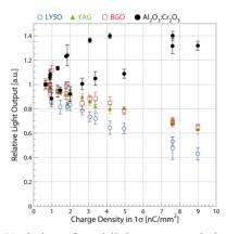
Figure 5: Variation of total light output and charge density at the screen position. The relative light output is normalized by total light output at the quadrupole strength of -14.03 T/m which corresponds to the start point of the quadrupole scan.
