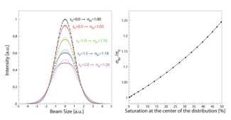
Figure 1: Saturation of the Gaussian distribution (a) and degree of over estimation of the beamsize as a function of the strength of the saturation at the center of the distribution. Solid lines in (a) show the Gaussian distributions fitted to the saturated data.
