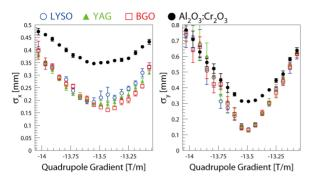
Figure 4: Horizontal and vertical beamsize (10 shots average) as a function of quadrupole strength.
