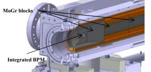
Figure 4: TCPPM-Jaw design with MoGr absorbing blocks and integrated BPM.
