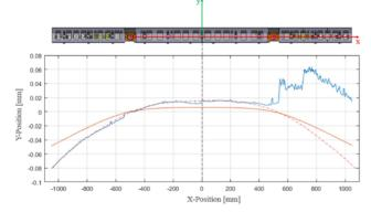
Figure 3: Comparison of the ANSYS® model (in red) and experimental prototype (in blue) of the TCDIL jaws.
