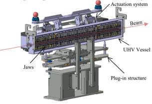
Figure 1: TCDIL collimator design.
