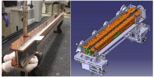
Figures 5 and 6: TCSPM prototype jaw with coated MoGr absorbing blocks and integrated BPM (left) and TCTPM collimator design (right).
