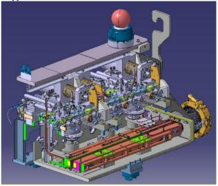
Figure 7: TCLD collimator design.
