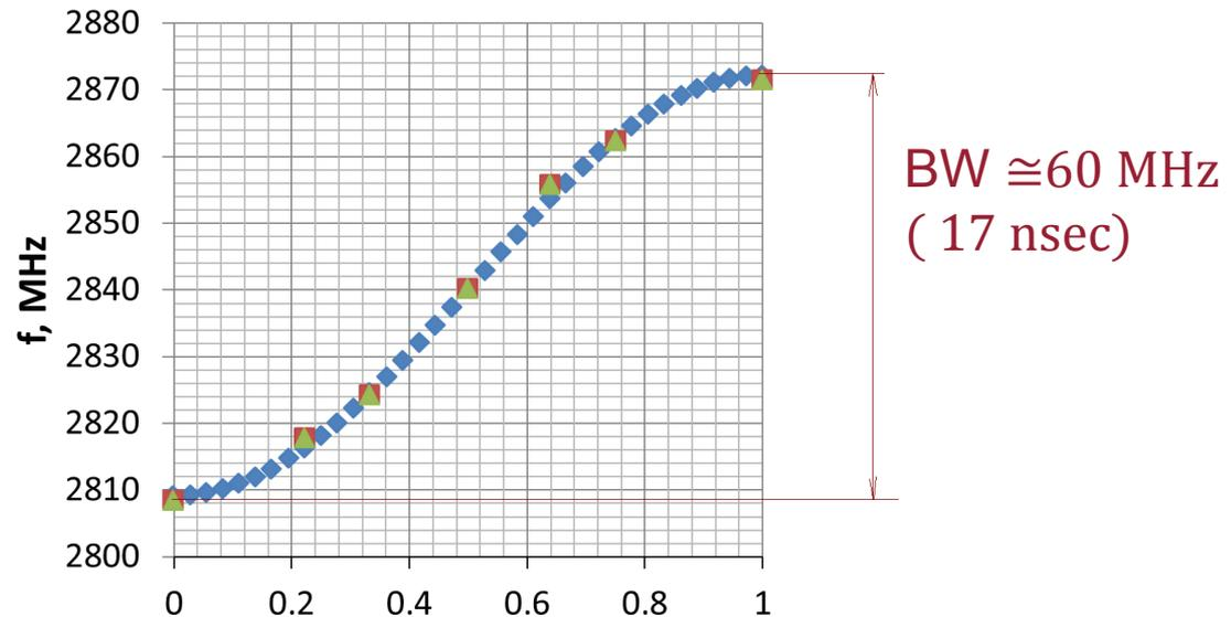
The BW of linac hardware (RF Source and Accelerating Structure) can be matched with the X-ray detector system based on modern X-Ray detectors
