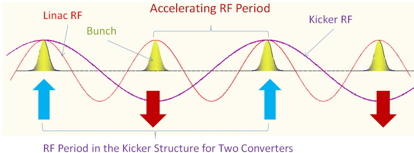
The natural frequency in the kicker structure is a sub harmonic frequency of the accelerating structure.
