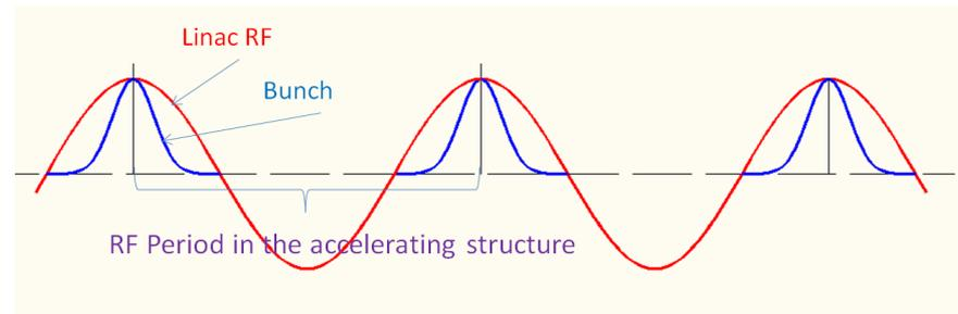
A bunched train is set at the crest of the RF amplitude. Each bunch gets a maximum longitudinal momentum.
