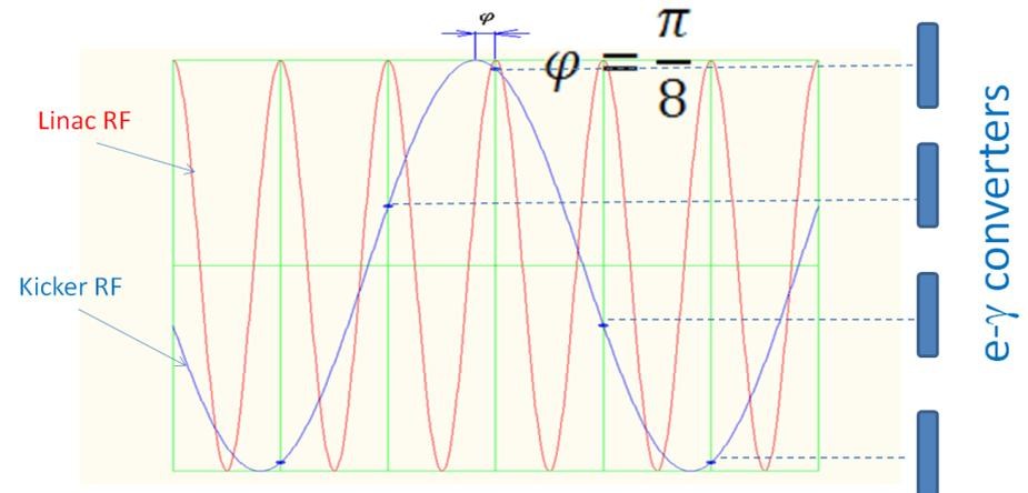
For example, S-band (2.856GHz) is a kicker RF frequency and X-Band (11.434GHz) is an RF frequency of the accelerating structure
