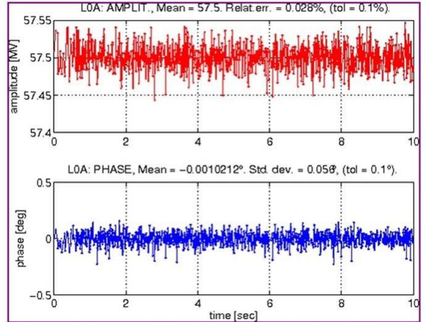
An RF amplitude stability of 0.03% with 0.06° STD of phase is demonstrated (at 2856 MHz and 120 PPS)
