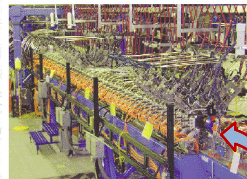
Figure 4. A halo channel photograph taken from the HEBT looking back toward the RFQ. The last four stations of wire-scanner, halo-scraper (eight units total) are visible on the right.
