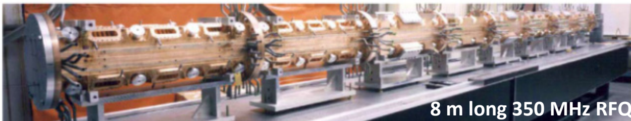
Fig. 10. The eight-meter-long RFQ of LEDA in the tuning stand.
