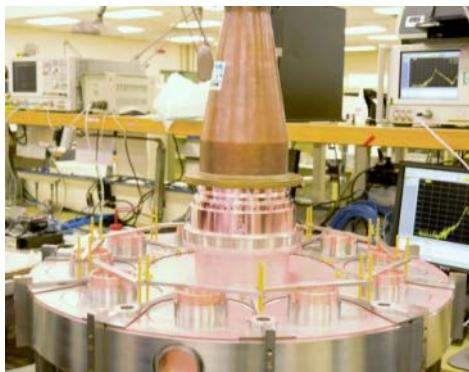
L3: Output cavity cold test
