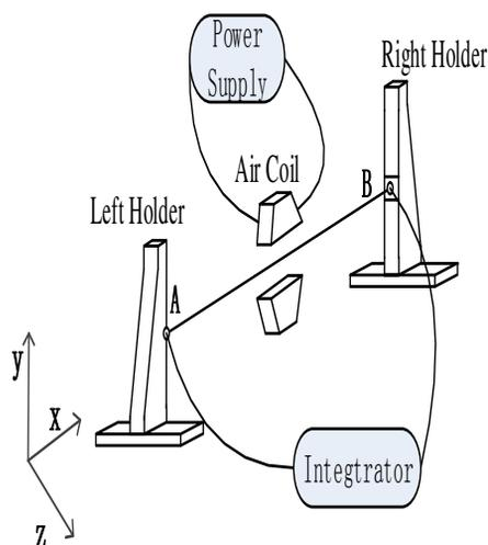
Figure 1: Schematic of the stretched wire system.
