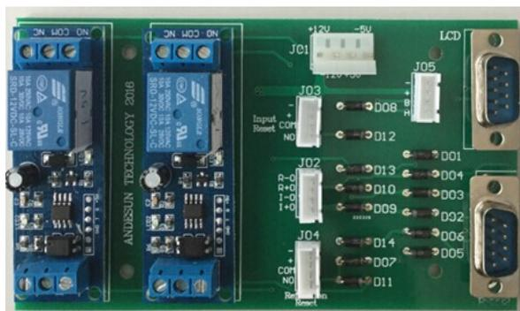
Figure 5: Control integrated-circuit-board developed by ANDESUN Inc.
