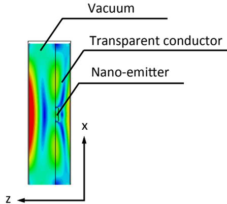
Figure 2: Simulation result of optical field distribution near the nano-scale photocathode.
