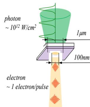
Figure 1: A schematic drawing of a nano-scale photocathode and photoemission. This method employs with a single electron per laser pulse, which completely removes the space charge effect.
