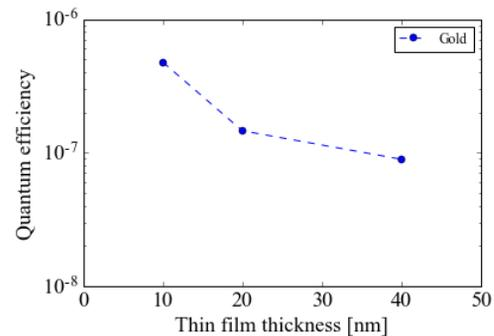
Figure 3: Measurement of quantum efficiency of gold thin film photocathode on  $\text{SiO}_2$ . This cathode was irradiated from the backside which avoid interference between the optical and electron paths.
