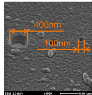
Figure 4: Focused Ion Beam (FIB) etched on multilayer. The scale bar corresponds to 400 nm.
