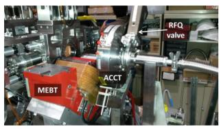
Figure 2: Assembly test of the ACCT.
