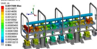
Figure 5: SRF Linac deformation after design optimization.
