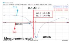
Figure 6: Measurement result on S parameter
