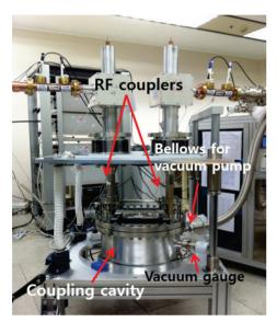
Figure 4: Test chamber assembled with RF couplers
