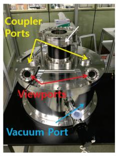
Figure 7: Coupling cavity for QWR RF coupler
