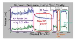
Figure 12: Vacuum state in pulsed mode
