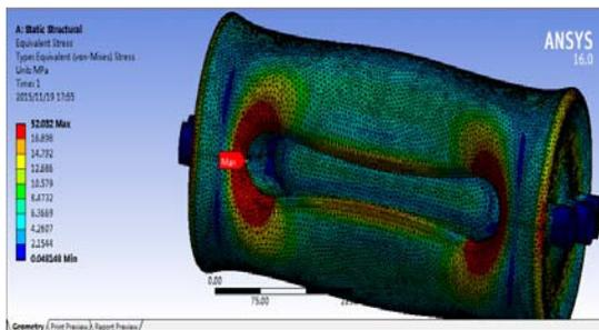
Figure 2: Stress of the bare cavity, got by ANSYS.
