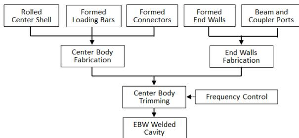
Figure 7: Fabrication procedure of the bare cavity.
