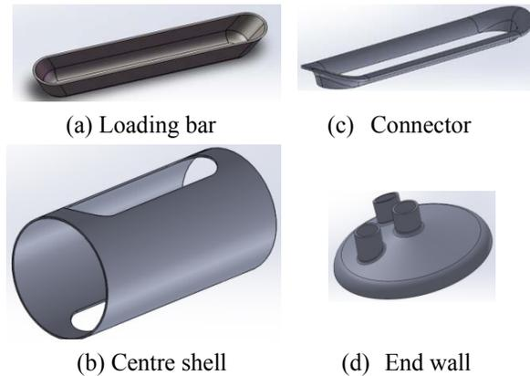
Figure 6: Main fabrication parts of the bare cavity.
