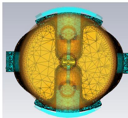
Figure 5: Cavity deformation due to Lorentz force.
