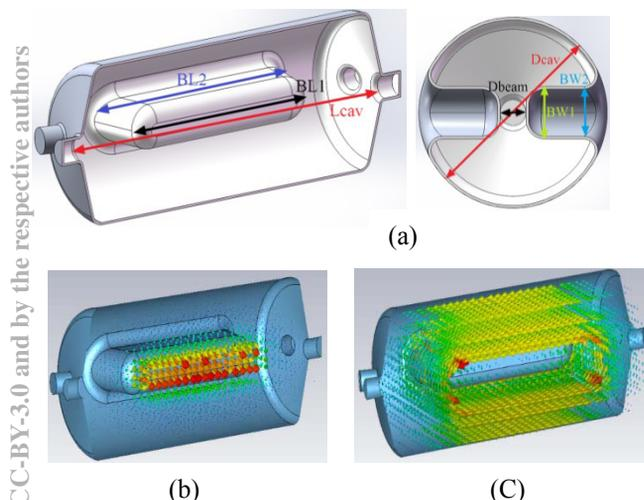
Figure 1: Geometrical parameters (a), electrical field (b) and magnetic field (c) of the deflecting cavity.
