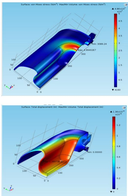
Figure 3: Stress (up) and deformation (down) distribution of the bare cavity, got by COMSOL.
