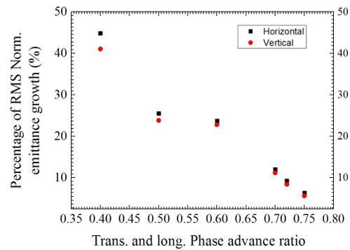
Figure 6: Maximum emittance growth percentages versus different phase advance ratios.
