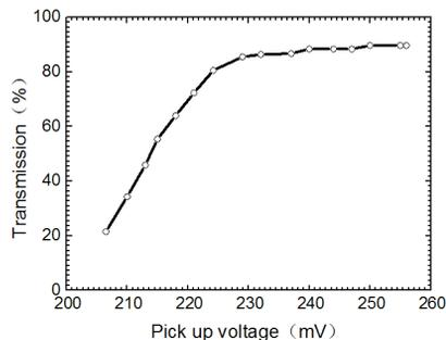
Figure 3: Verification of tank level with transmission scan.
