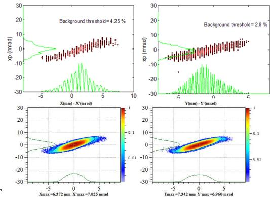
Figure 7: Measurement emittance results by two slits at the exit of CM1 (upper graph) comparing with the simulation results (below figure).
