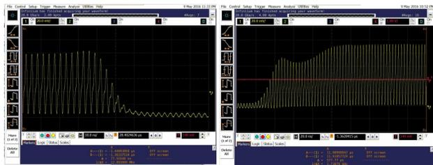
Figure 2: LEBT chopper rise time (left trace) and fall time (right trace) measured at the MEBT FCT.
