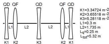
Figure 6: Emittance exchange with 5 skew quadrupole magnets.
