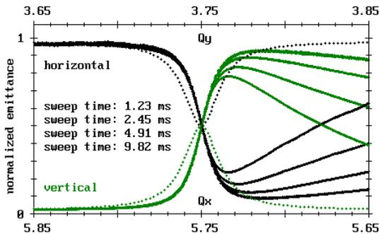
Figure 3: Variation of the normalized emittances as the tunes are swept across the linear coupling resonance with increasing speed. The coupling strength is constant and for very slow sweeps the dotted, theoretical curve would be obtained, similar to Fig. 2. The horizontal axis is also the time axis with the indicated full sweep time. Time increases from left to right.
