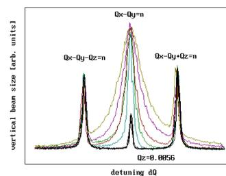
Figure 2: Vertical beam size close to the coupling resonance for decreasing coupling strengths. On resonance the emittance reaches a value independent of coupling above a certain coupling strength.
