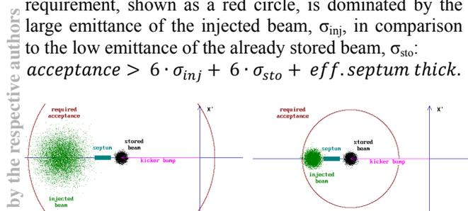
Figure 1: Impact of the injected beam emittance on the aperture requirement.
