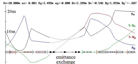
Figure 7: BESSY II transfer line optics with emittance exchange by 5 skew quadrupole magnets. The creation of vertical dispersion and the horizontal dispersion produced further downstream turn this scheme useless. The Twiss parameters at the end of the transfer line are shown at the top.
