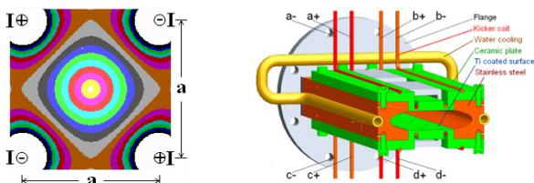
Figure 5: left – wire arrangement for producing pulsed skew gradient fields, right – sketch of our non-linear injection kicker magnet where the currents in all wires flows in the same direction and return wires further out are needed.
