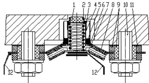
Figure 4: Layout of the microtron cathode assembly. 1-emitter, 2- graphite holder, 3- cathode sleeve, 4- cylindrical filament , 5- heat shields, 6- carrying base, 7-
