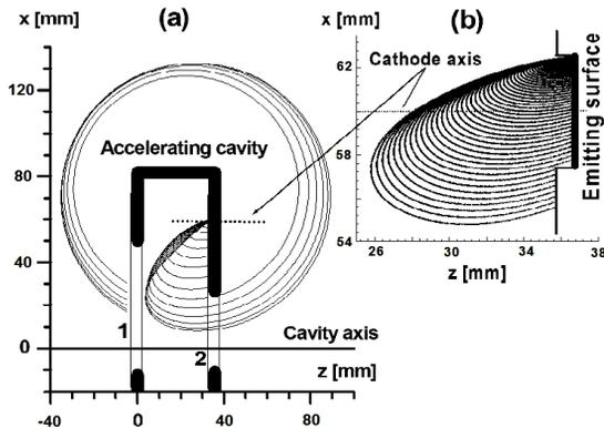
Figure 3: (a) 2-D tracking of the first orbit. With numbers 1 and 2 are marked the narrow slits directed along the  $x$  axis and used for input-output of the electrons. (b) 2-D
