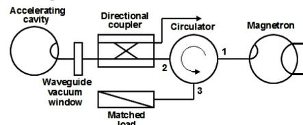
Figure 1: Conceptual scheme of the microtron RF system
