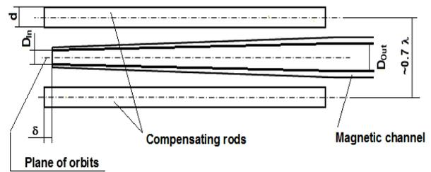
Figure 6: The extracting system of the L-band microtron.
