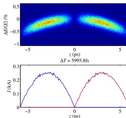
Figure 2: The initial longitudinal phase space of the two bunches at the beginning of L1. The initial time separation is 6 ps. The blue line is for the head bunch and the red one is for the tail.
