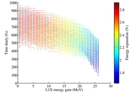
Figure 7: Correlations between L1X energy gain and the time delay and energy separation. The initial delay is 6 ps.
