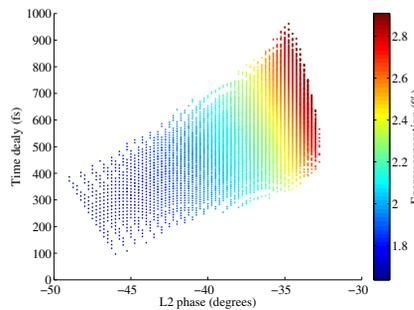
Figure 6: Correlations between the L2 phase and the time delay and energy separation. The initial delay is 6 ps.
