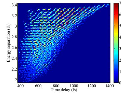
Figure 8: The distribution of time delay and energy separation with peak current of core part >10 kA. The initial time delay of the two bunches is 10 ps.
