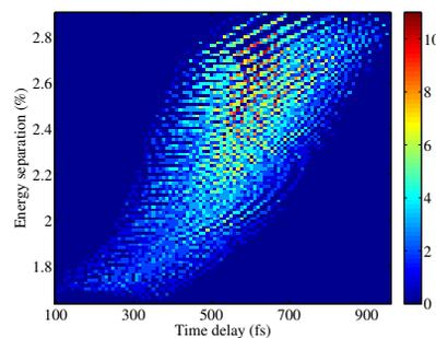
Figure 3: The distribution of time delay and energy separation of the two bunches with peak current of core part >10 kA in the simulation scans. The initial time delay of the two bunches is 6 ps.
