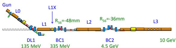
Figure 1: A schematic layout of the twin-bunch method in a double-chicane beamline (not to scale).
