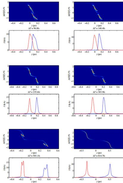
Figure 4: Phase spaces with different time delays from ~100 fs to ~800 fs. The initial delay is 6 ps.
