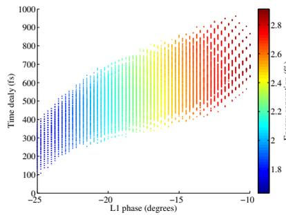
Figure 5: Correlations between the L1 phase and the time delay and energy separation. The initial delay is 6 ps.
