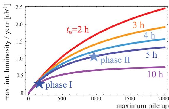
Figure 2: Maximum integrated luminosity per year as a function of maximum pile-up, assuming 160 days of physics run, a machine availability  $A$  of 71%, two primary collision points ( $n_{\text{IP}} = 2$ ),  $n_b = 10600$  bunches per beam, and a maximum beam intensity of  $N_{b,0} = 10^{15}$  protons. The various curves correspond to different average turnaround times  $t_{\text{ta}}$ . The design working points for FCC-hh Phases I and II [3] are also indicated.
