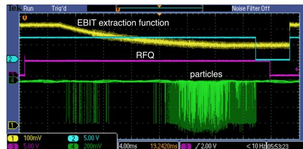
Figure 2: Particle distribution ( $^{78}\text{Kr}$ ) extracted from the EBIT and detected in the experiment.
