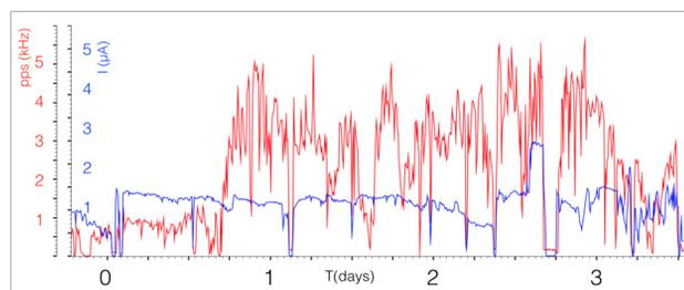
Figure 3: Beam intensity of rare isotope  $^{37}\text{K}$  in the experimental set-up (red curve) together with the primary beam intensity of  $^{40}\text{Ca}$  beam (blue curve) provided by the Coupled Cyclotrons of NSCL .
