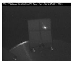
Figure 4:  $^{37}\text{K}$  measured beam spot in the target of the experiment. The beam intensity is 1000 pps and timing macro-structure of 2Hz. The size of the spot is 2mm.
