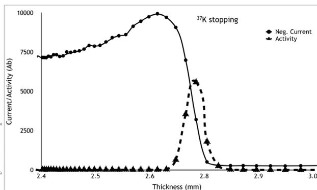
Figure 1: Negative current in the front window of the gas cell (solid curve) and beta activity detected after the gas cell (dashed curve) as a function of the total degrader thickness. See text for details.
