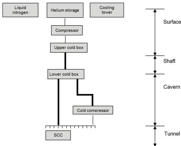
Figure 3: General architecture of the CEPC cryogenic system.
