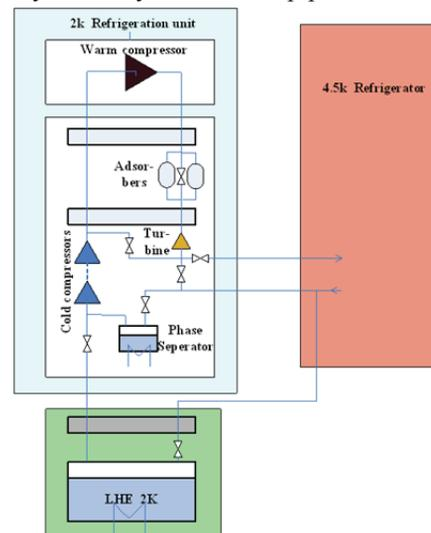
Figure 2: 2 K refrigerator flow diagram.
