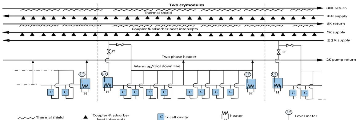
Figure 4: The flow scheme of CEPC collider ring.
