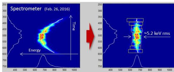
Figure 4: Example of a longitudinal phase space measurement for a 22 pC, 3.2 A peak current and 15.7 MeV beam. Left: full phase space. Right: phase space after removal of 1<sup>st</sup> and 2<sup>nd</sup> order correlations.
