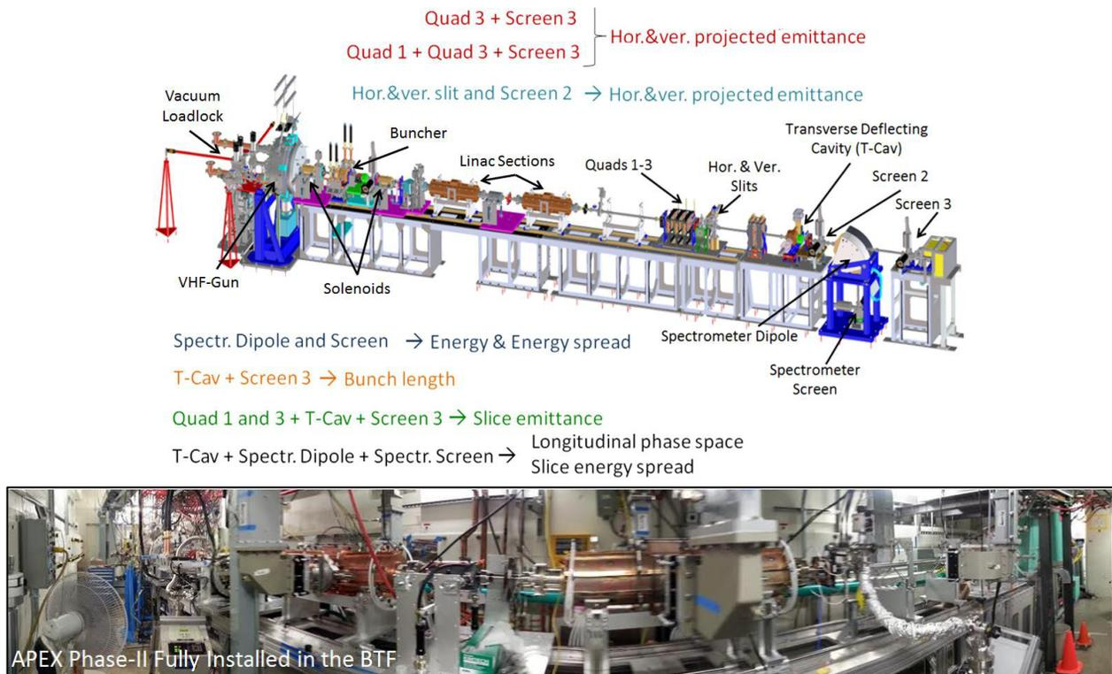
Figure 1: APEX Phase-II beamline. Top: CAD view. Bottom: panoramic photo of the beamline.
