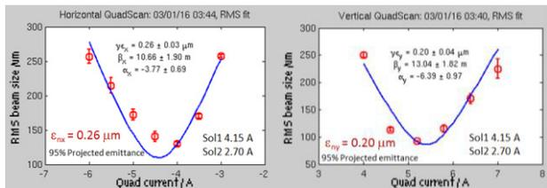
Figure 2: Example of a 95% projected emittance measurement for a 20 pC, 6.5 A peak current and 15.7 MeV beam.
