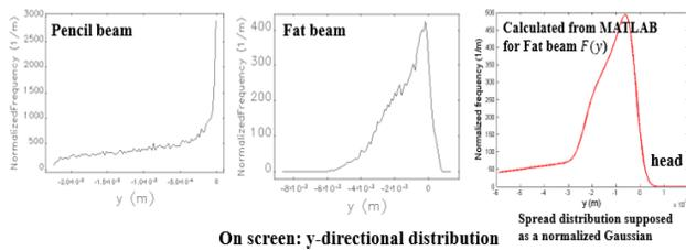
Figure 5: y-directional distribution on the screen. Left is pencil beam, middle is fat beam and right is calculated ( $y$ ) with assumed as normalized Gaussian of spread distribution.
