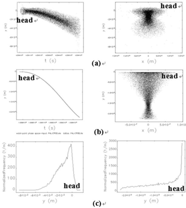
Figure 3: ELEGANT simulation results, t-y plane (left of (a) and (b)) and x-y plane (right of (a) and (b)) projection on screen. (a) Fat beam. (b) Pencil beam. (c) y-directional distribution on screen of fat beam (left) and pencil beam (right)
