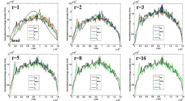
Figure 4: The Reconstruction method outputs. Initial longitudinal beam distribution is uniform-ellipse. r is iteration cycles of reconstruction and  $I_0$  is original current.
