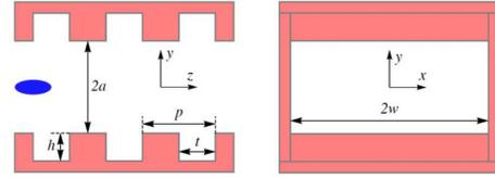
Figure 1: Geometry of dechirper parameters. Side (left) and front view (right) of the dechirper.
