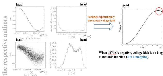
Figure 6: Left pictures are pencil and fat beam side view and y-directional distribution on the screen. Right picture is particles experienced voltage kick.
