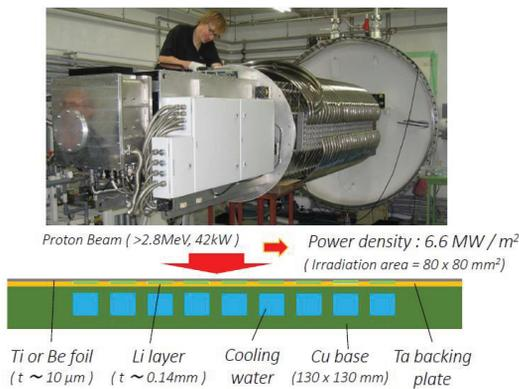
Figure 7: Picture of the Dynamitron (upper) and cross sectional drawing of the target (lower) [2].
