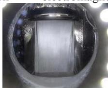
Figure 9: Liquid Li flow in the circulating loop (from top to bottom) [6].
