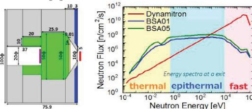
Figure 8: A cross sectional drawing of the moderator and estimated neutron spectrum at the exit of the dynamitron (red), original moderator design (blue) and improved design (green).
