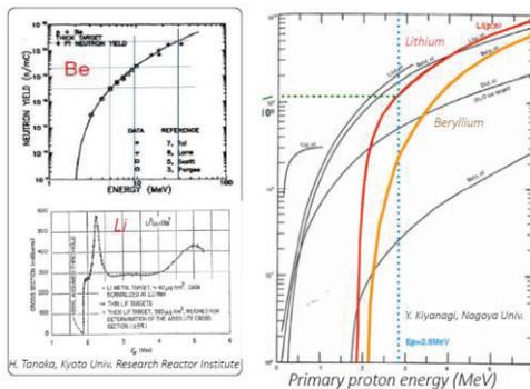
Figure 3: Comparison of neutron production cross-sections for Be and Li as a function of primary proton energy [2].
