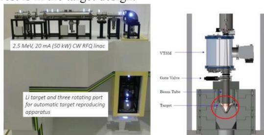
Figure 6: Schematic drawing of the NCC facility configuration (left) and target system with automatic Li layer reproducing apparatus (right) [5].
