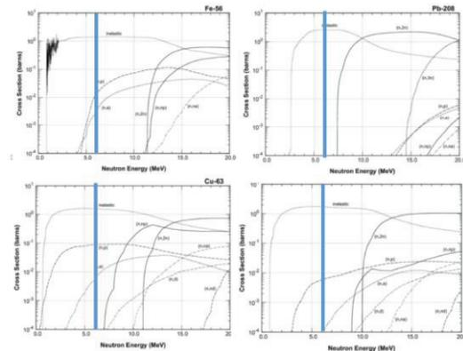
Figure 10: Nuclear reaction cross sections (barns) for  $^{56}\text{Fe}$  (upper left),  $^{208}\text{Pb}$  (upper right),  $^{63}\text{Cu}$  (lower left) and  $^{65}\text{Cu}$  (lower right) as a function of neutron energy [8]. Blue vertical lines are at 6.1 MeV.
