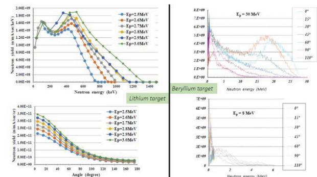
Figure 4: Neutron energy spectrum for various production angles for Li (left) and Be target (right) [2].
