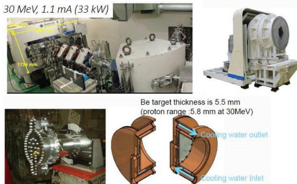
Figure 5: Photos of the cyclotron (upper left), moderator (upper right) and target system (lower) [3]. The Be is 5.5 mm in thickness, which is slightly thinner than the Bragg peak depth of the beam. The beam is stopped in the cooling water layer which resolves the blistering problem.
