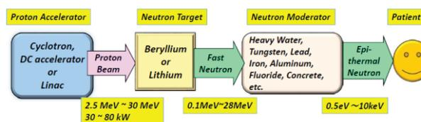
Figure 2: Block diagram of an accelerator-based BNCT facility.
