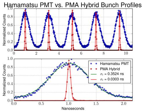
Figure 2: Bunch profile comparison of the Hamamatsu H3760-01 vs PicoQuant Hybrid-06 PMA detectors. The H3760-01 initially in service was not designed for this application.
