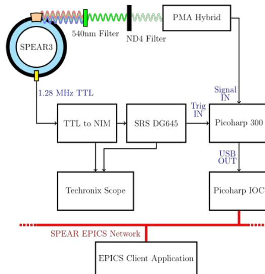
Figure 1: Block diagram of the TCSPC hardware and signal layout
