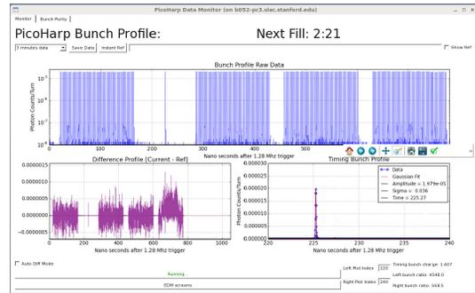
Figure 3: GUI layout for control room monitoring of bunch trains, timing bunch fitting, and new fill difference profile.
