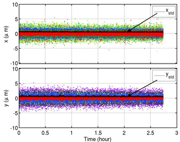
Figure 4: The orbit stabilization of the HLS-II storage ring. All the BPM values and the rms orbit value over all BPMs are plotted as a function of time.
