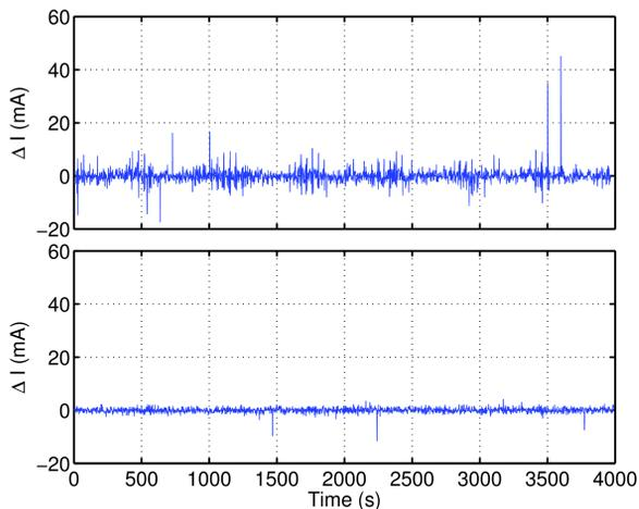
Figure 5: The stability of the PS output at fixed setpoints. (up) before optimization; (down) after optimization.
