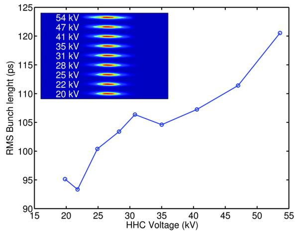
Figure 3: Beam bunch stretching using the 4th harmonic RF cavity.
