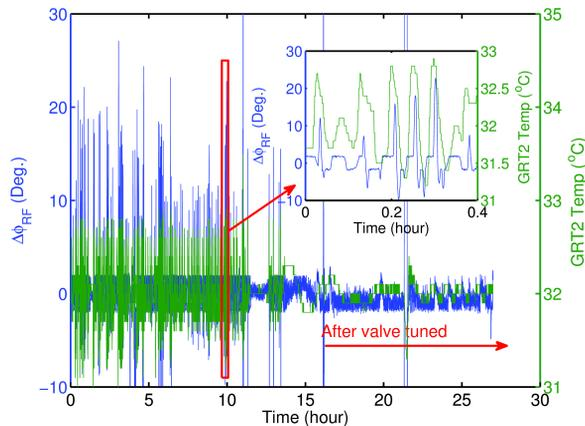
Figure 7: Impact of the water cooling system on the phase stability of the RF cavity.
