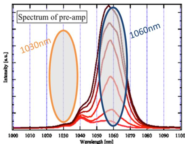
Figure 5: Amplification in 1060nm with Yb-doped single mode double clad fiber [3].
