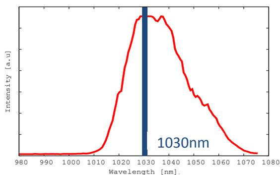
Figure 4: Spectrum of pulse from oscillator.
