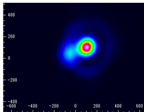
Figure 6: Spatial beam profile of pulse from PCF amplifier.
