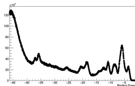
Figure 5: An example of CsK<sub>2</sub>Sb UPS spectra.
