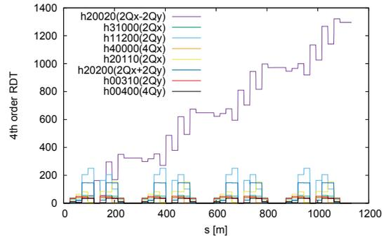
Figure 5: 4rd order resonance driving terms due to sextupoles in ARC (24cells).
