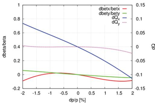
Figure 3: Chromatic functions at IP with the IR only (one side).
