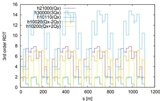
Figure 4: 3rd order resonance driving terms due to sextupoles in ARC (24cells).
