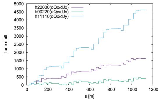
Figure 6: Tune shift due to sextupoles in ARC (24cells).
