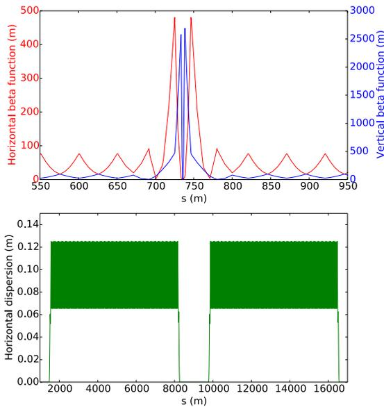
Figure 1: Optics at the IP for the 12 folds lattice at 120GeV.
