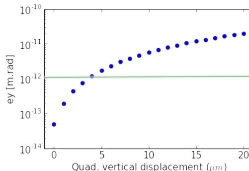
Figure 7: Resulting vertical emittance after dispersion free steering and chromaticity correction as a function of transverse displacement into the quadrupoles at 175GeV.
