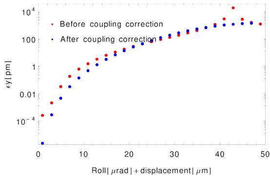
Figure 2: Emittances as a function of roll and displacement errors into the lattice.
