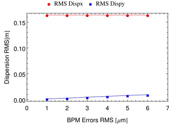
Figure 4: Resulting RMS vertical dispersion with BPM error readings.
