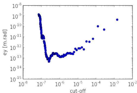
Figure 6: Resulting vertical emittance after dispersion free steering and chromaticity correction as a function of the number of singular values taken into account into the system.
