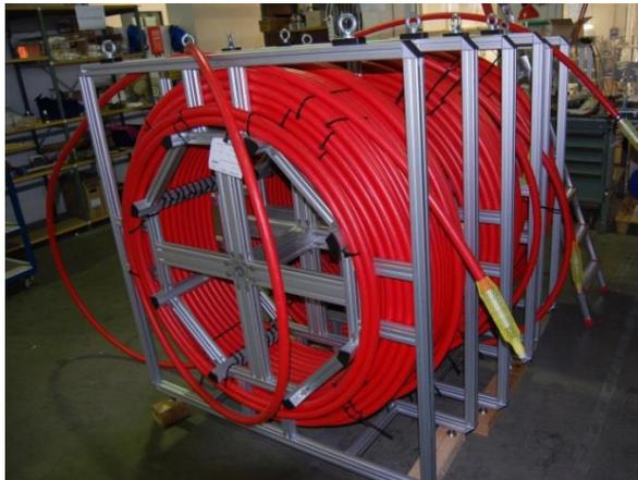
Figure 4: Cable drums for energy storage cables.
