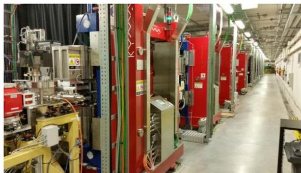
Figure 3: FEL-2 with the new installed EPU.
