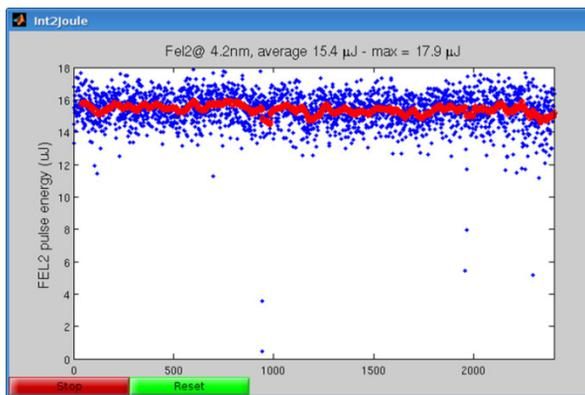
Figure 4: FEL-2 pulse by pulse intensity at 4.2 nm.
