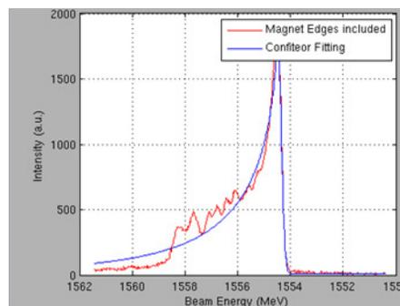
Figure 2: Maximum LINAC operating energy.
