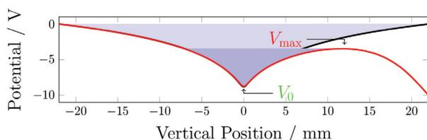
Figure 2: Vertical beam potential at 1.7 GeV and 50 mA, superimposed by the local potential of the HVCE, positioned at 22 mm, biased with  $-10$  V (red) and  $0$  V (black).
