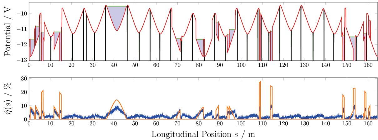
Figure 3: Top: Estimated beam potential depth at 1.7 GeV and 50 mA along the stretcher ring (red) with superimposed  $-3$  kV-HVCE potential (black). The SC modified potential due to ion accumulation in potential wells is shown in green. Bottom: The local neutralisation  $\hat{\eta}_{\text{stat}}(s)$  along the stretcher ring is shown in orange and  $\hat{\eta}_{\text{dyn}}(s)$  in blue.
