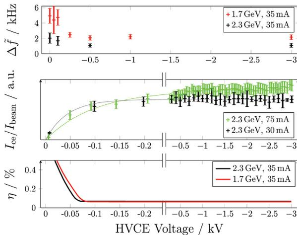
Figure 4: Top:  $\Delta f$ -Parameter for different HVCE voltages derived from BTF measurements. Middle: Normalized HVCE current for different beam currents with corresponding fits. Bottom: Theoretical prediction on  $\eta$ , summing up  $\eta_{\text{stat}}$ ,  $\eta_{\text{ce}}$  and  $\eta_{\text{dyn}}$ .
