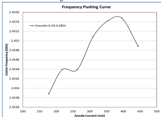
Figure 6: Frequency push curve by anode current change.
