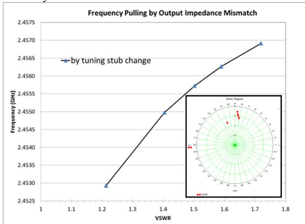
Figure 7: Preliminary frequency pulling curve measured by one stub change only on the output waveguide.
