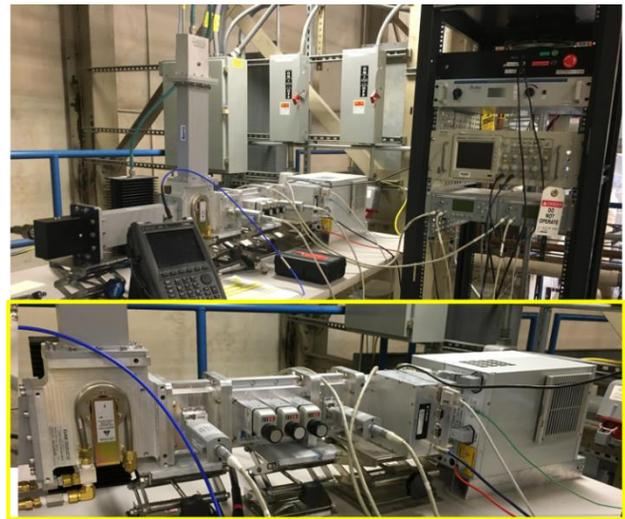
Figure 1: 2.45GHz, 1.2kW magnetron test stand (top) and the setup (bottom) connected to a matched load.
