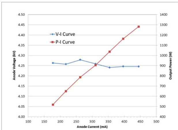
Figure 4: V-I and P-I curves of TMA12 magnetron.
