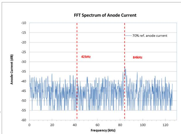
Figure 8: FFT spectrum measured directly by TDS2014B scope from magnetron power supply anode current monitor.
