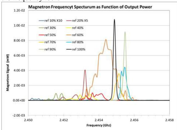
Figure 3: MKS TMA12 magnetron power spectrum measurement to a matched load through a WR340 coupler.
