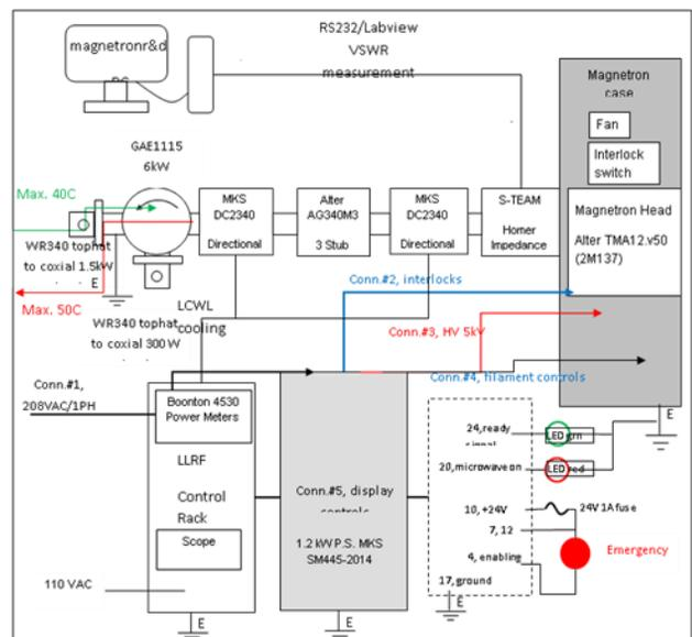
Figure 2: Circuit diagram of Alter magnetron test to a matched load for Rieke diagram measurement.
