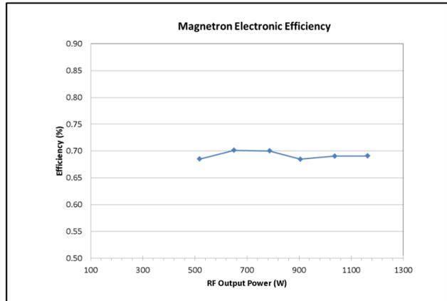
Figure 5: Electronic efficiency in operation parameter range.
