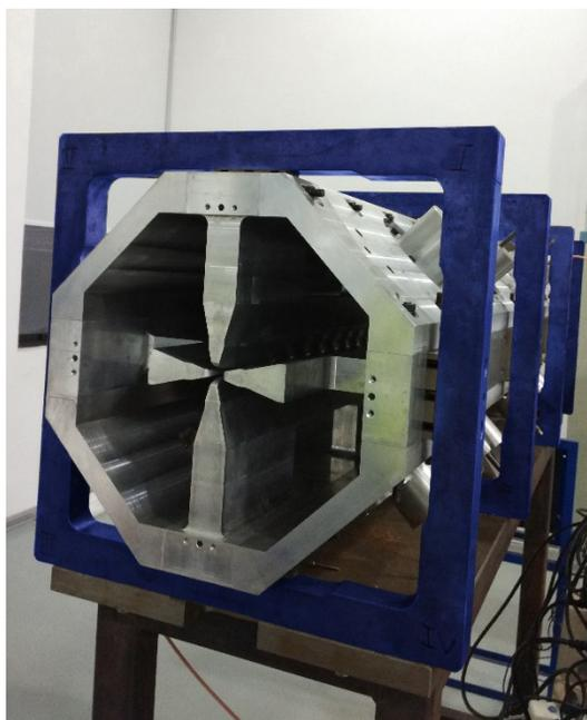
Figure 5: Aluminium RFQ prototype with open cavity.
