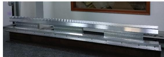
Figure 4: One of the modulated vanes.
