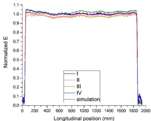
Figure 6: Normalized inter-vane electric field along the RFQ for 4 quadrants. Simulated result acts as contrast.
